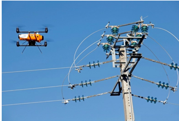
Figure 1.2.4.b - A figure representing a civil drone exploited to inspect electric lines.
